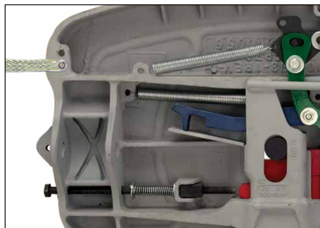
Figure 4: On fifth wheels with manual pull handle release, connect ground strap using same directions as Figure 3.
