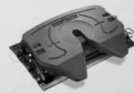
H7 Blocked PS5 Stationary 70,000 lbs vertical load 200,000 lbs drivebar pull
